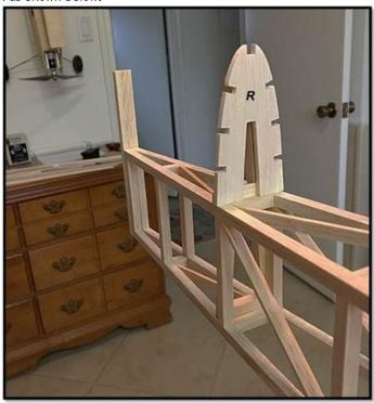
1/16" spacers were put in between the R bulkhead and the A-Frame when they were glued together in order to center the 1/8" R bulkhead over the 1/4" vertical upright as you see below. I had serious concerns over the stab platform's narrow width available to mount the removable stab illustrated in green below.
