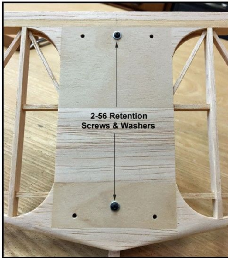
The fin/stab assembly was attached to fuselage's stab platform for a trial fit.
