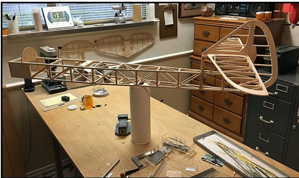
The fin was attached to the stab which was then mounted on the fuselage's stab platform. The rudder was attached to the fin with the continuous hinge pin wire as shown below.
