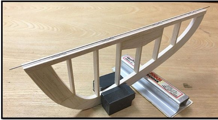
This picture shows the rudder attached to the fin with a continuous hinge pin wire.
