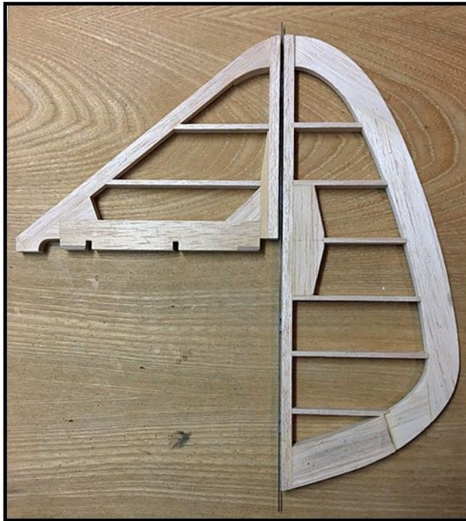
This picture shows the rudder attached to the fin with a continuous hinge pin wire.
