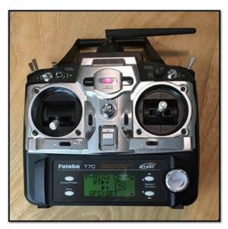
Now as the throttle is advanced from zero to the mid-point, the down elevator deflection goes from zero to 12% at the mi-point and then from 12% to 35% from the mid-point to full on as shown below. While this not exponential, it is two linear mixes with a shallow slope first and then a steep slope.
