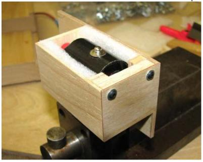
This shows the unit bolted to back of the SP's firewall. Notice the clearance cut outs in the unit's base for the T-Mounts 6-32 blind nut flanges on the back of the firewall. Notice also the larger hole in the removable end that secures the coil in the unit's coil compartment.
