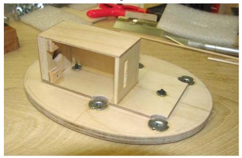
The wood on this unit was given five coats of clear doped to seal all of its surfaces. Then Velcro was applied to back side of the unit's coil compartment for shock mounting Marv Stern's Aero Tech IGN-SW ignition module and to the unit's base in front of the coil compartment for shock mounting the 3-cell ignition battery as shown below.
