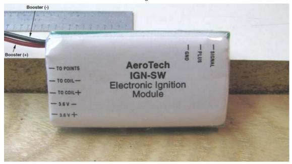
This is a nice shot of the Aero Tech IGN-SW ignition module and the 3-cell ignition battery installed on the unit and partially wired up.
