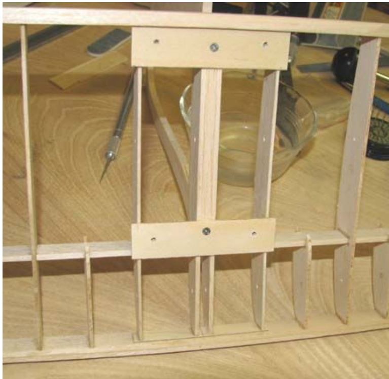
This shows a close up of one of the 2-56 countersunk screws.
