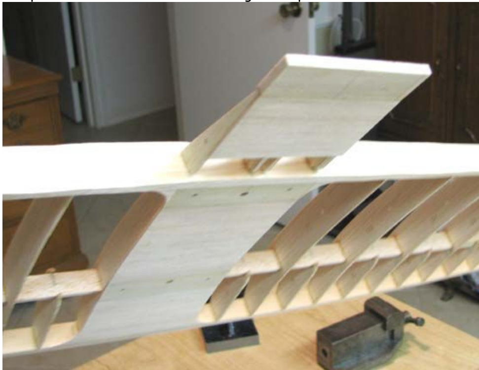
This shows the fixed portion elevator's center section glued in place on the back of the stab's rear spar.
