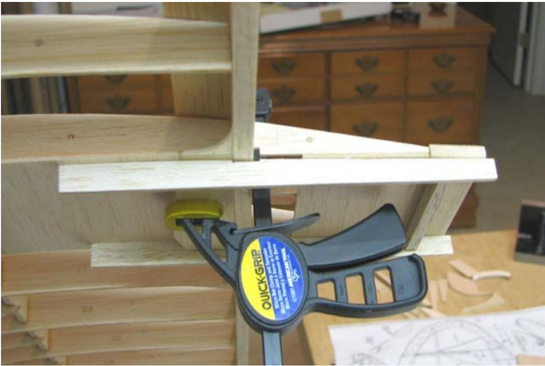
This shows the fixed portion elevator's center section glued in place on the back of the stab's rear spar.
