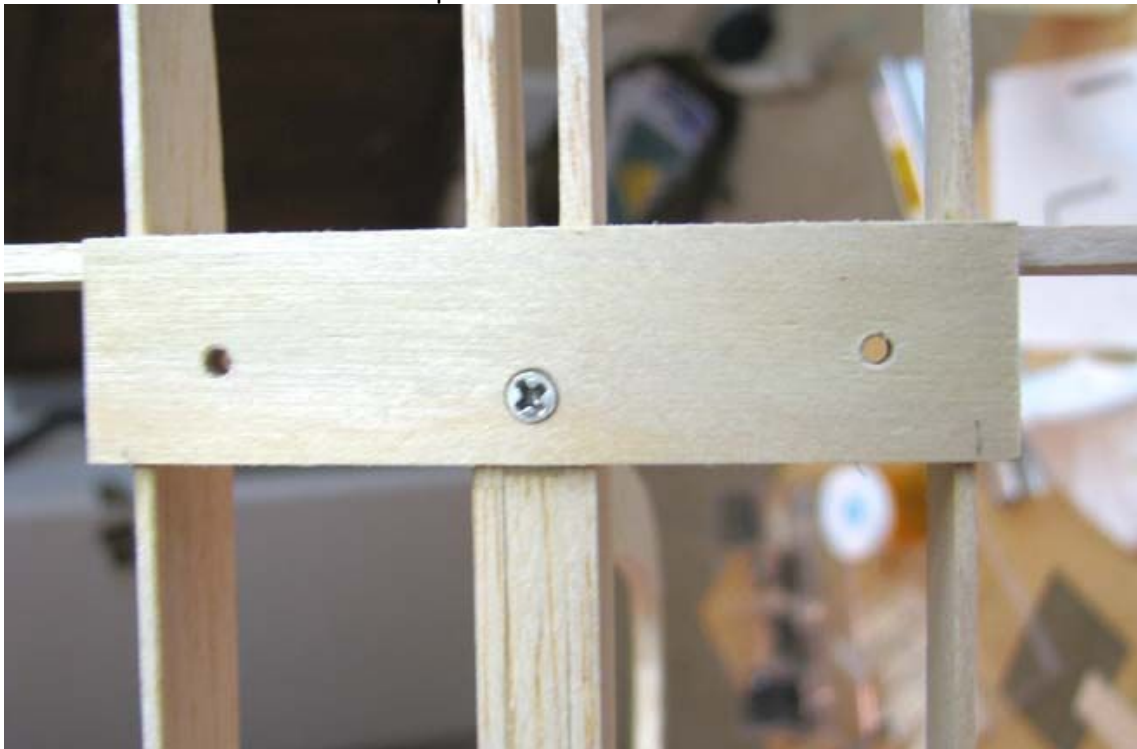
This shows a close up of one of the 2-56 countersunk screws.
