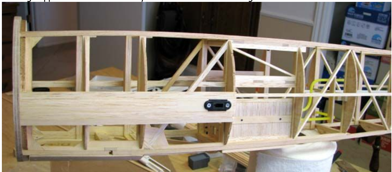
This picture shows the Ernst charging jack installation from the outside. The jack is located on the left side of the fuselage opposite where the McCoy 60's exhaust will discharge.
