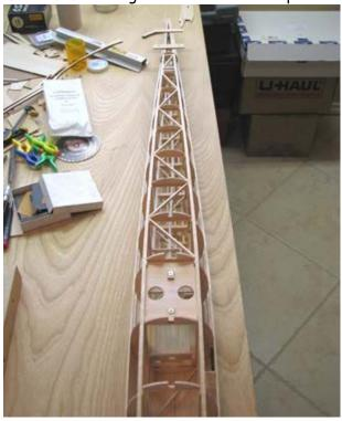
This shows how the top diagonals run in the opposite direction to bottom diagonals.
