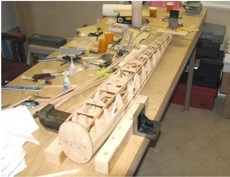
This picture shows a close up of both the clamping and weighting used on the center segment of the stab platform 1/8" balsa sheeting between the two 1/8" plywood stab mounts.
