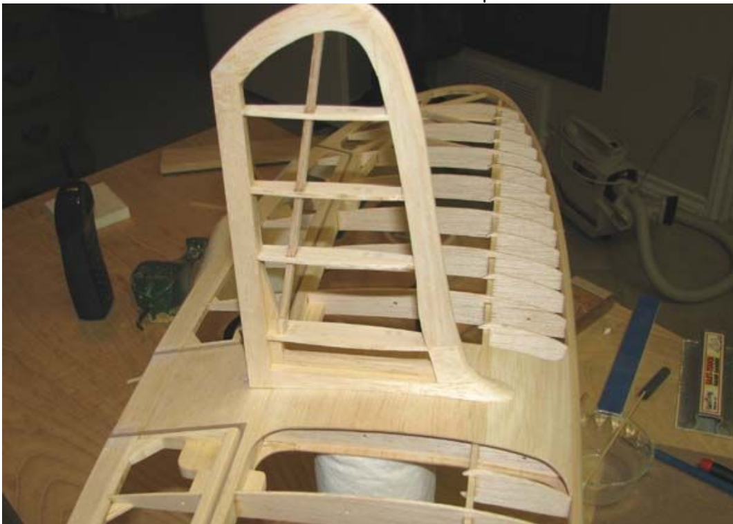
This shows the fin mounted in the stab slot. Notice the shape of the fin's forward fillet now.
