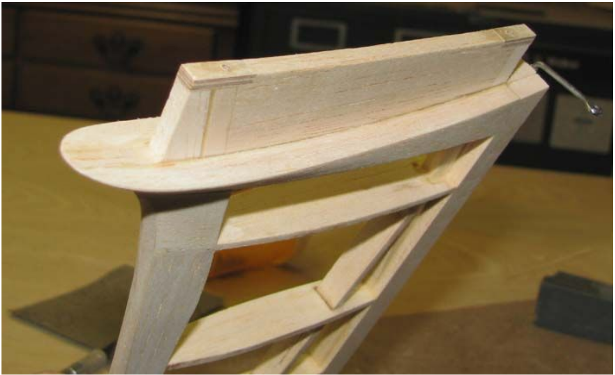
This shows the fin mounted in the stab slot. Notice the shape of the fin's forward fillet now.
