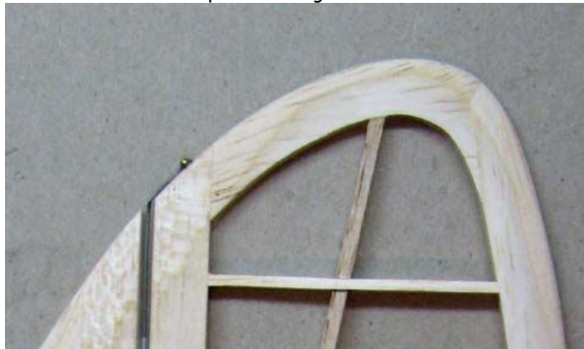
This is a close up of the hinge wire retention screw.
