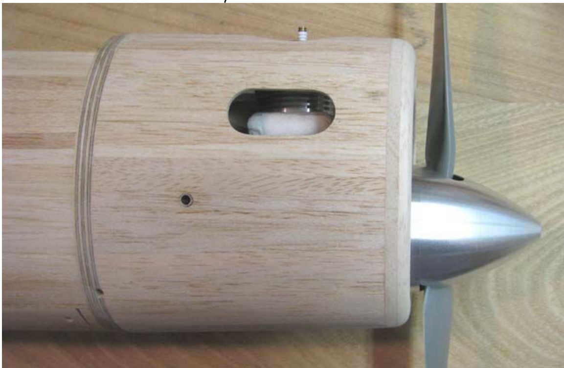
The 0.27" prop drive spool length Woody made for me provides the perfect prop clearance relative to the front of the cowl as shown below.....Tandy
