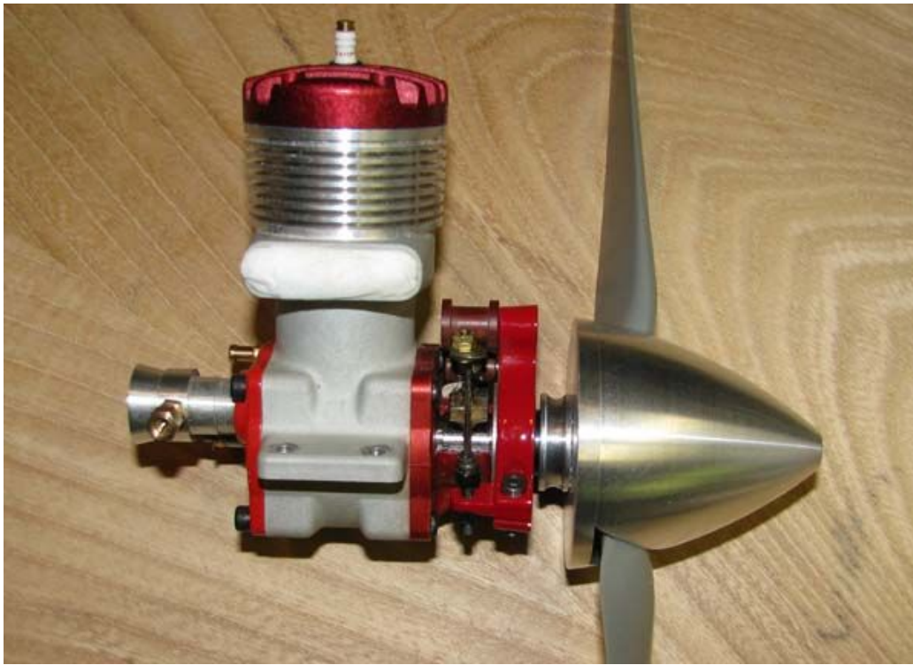
The 0.27" prop drive spool length Woody made for me provides the perfect prop clearance relative to the front of the cowl as shown below.....Tandy
