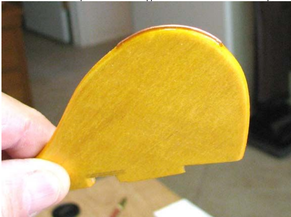
This is a close up of one of the copper wires CA'd to the sub fin tip.
