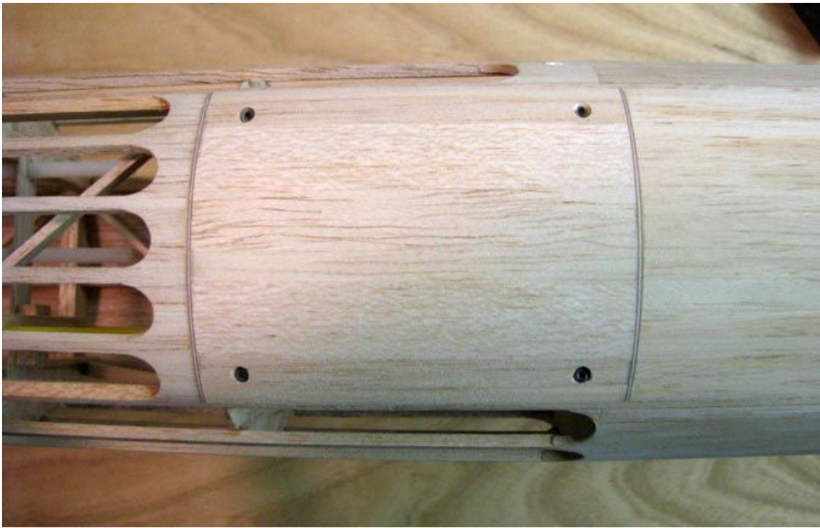
Finally, this shows both the fore and aft hatch covers installed completing the bottom of the Sailplane fuselage.....Tandy
