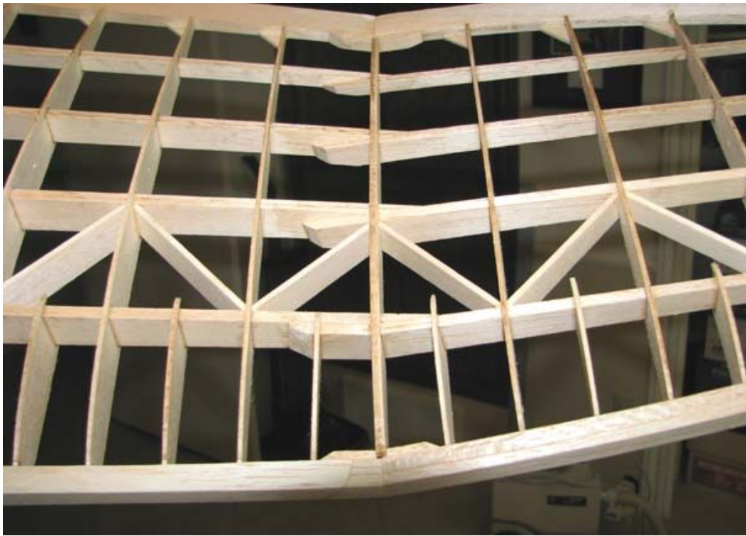
This is a second view of the completed polyhedral joint from the bottom.....Tandy
