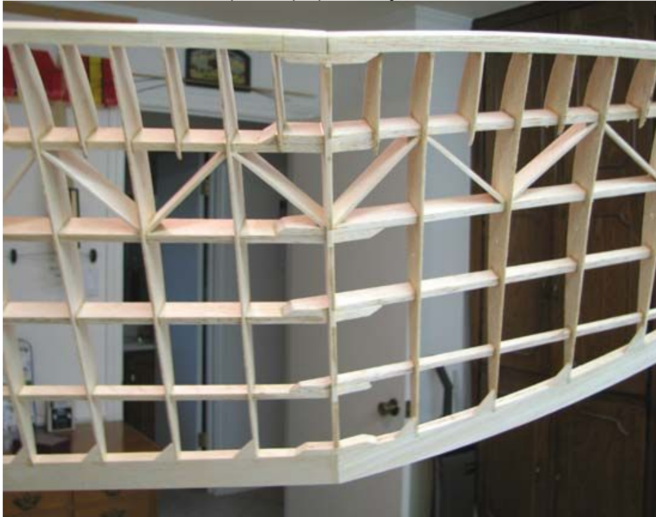
This is a second view of the completed polyhedral joint from the bottom.....Tandy
