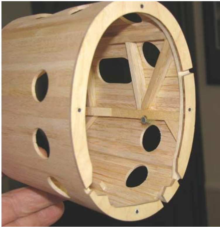
This bottom view shows the three holes in the bottom of the cowl.
