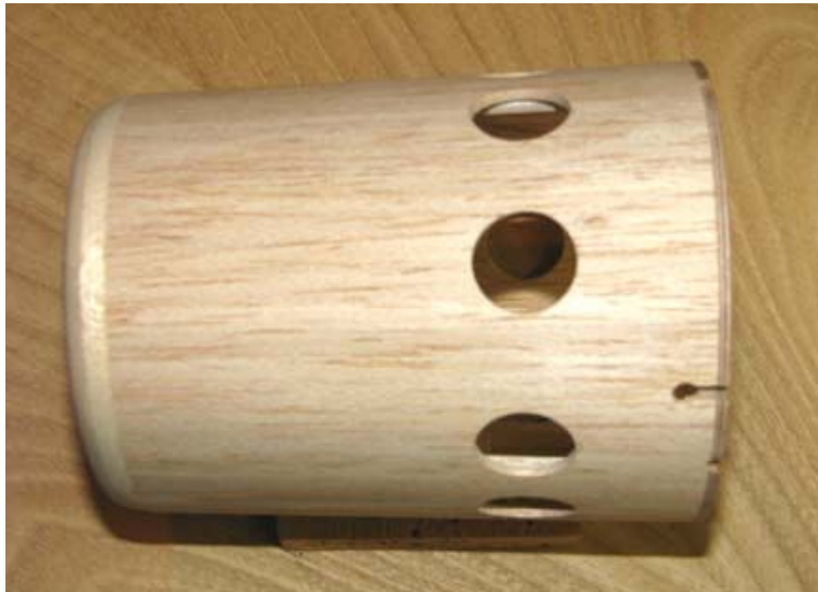
This bottom view shows the three holes in the bottom of the cowl.
