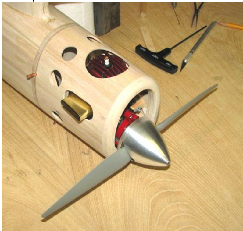
This shows the completed installation of the brass exhaust extension.....Tandy
