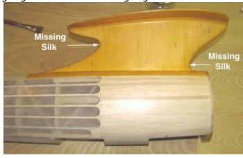
This close up is an attempt to show the area void of silk in the neck of the leading edge. The color in this picture is significantly off due to the lighting and no flash.
