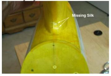
I tried cutting a small patch of raw orange silk and clear doping it over the missing area several times, but I kept ending up in a mess. The raw silk would distort and bunch up. I had to take Acetone and remove the silky glob! So I got the idea of predoping the silk so it would hold its shape while being applied. I keep a frame around for experimentation. I covered a bay of the frame and clear doped it several times as shown below.
