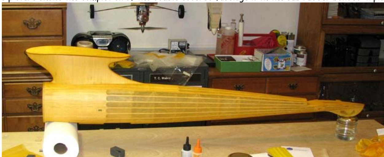
This picture shows the completion of the double covered fuselage with the sub rudder bonded in place.
