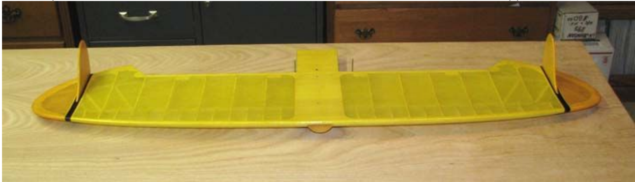
This is a picture of the bottom of the stab with the two removable sub fins slipped into their slots.
