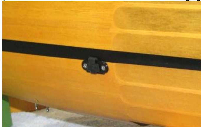
This picture shows a left side view of the Ernst charging jack.
