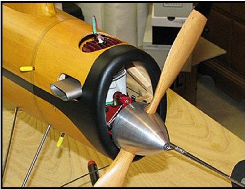
This picture shows the exhaust extension held securely in place on the engine with springs inside the cowl.
