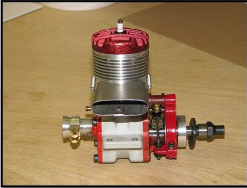
This picture shows the exhaust extension held securely in place on the engine with springs inside the cowl.
