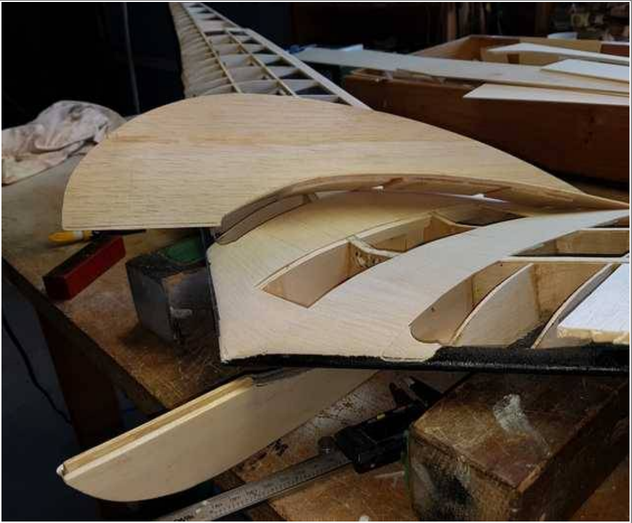
Rx and battery access from the top removable central fin, in my case held in place by 2 magnets.
