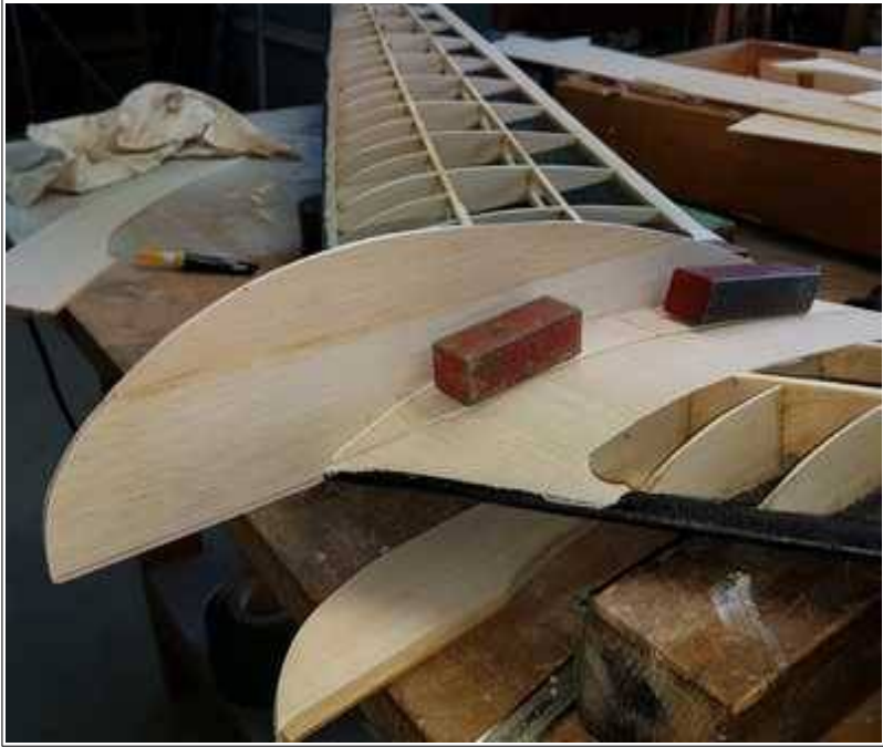
Rx and battery access from the top removable central fin, in my case held in place by 2 magnets.
